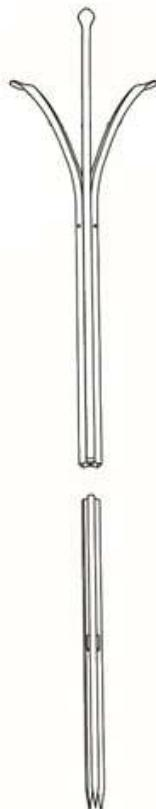
Step 4: After all the legs are held together with their montage pieces (**E**) and screws (**F**) slip the open end over the exposed stakes that you drove into the ground earlier.
