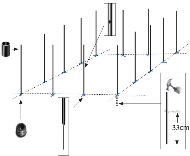
Make a pilot hole to the depth marked on the hole-make.
